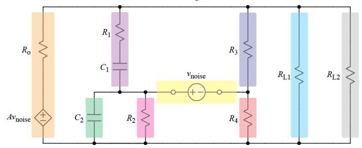
Components in the same branch are in series:  $R_0$  and  $Av_{\text{noise}}$  are in series, and  $R_1$  and  $C_1$  are in series. Non-essential nodes separate components in series, (see CONCEPTUAL TOOLS: CIRCUITS: CONFIGURATION: Identifying Nodes).
