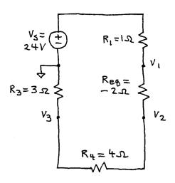
Now we can use v-divider egins to find  $V_1$ ,  $V_2$ , and  $V_3$ :
