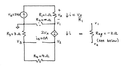
We observe that current  $i = v_x/R_1$  flows thru  $R_1$ , creating  $v_x$ , and thru the dependent source, creating -xvx. Thus, we may replace the dependent source with an equivalent R:
