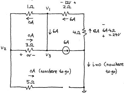
All the current will flow thru the wire between  $v_i$  and  $v_3$ , (path of least resistance).
