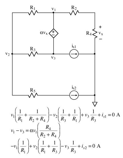
Make a consistency check on the above node-voltage equations for the circuit by setting resistors and sources to values for which the values of  $v_1$ ,  $v_2$ , and  $v_3$  are obvious. State the values of resistors, sources, and  $v_1$ ,  $v_2$ ,  $v_3$  for your consistency check, and show that the node-voltage equations are satisfied for these values. (In other words, plug the values into the node-voltage equations and show that they yield values of zero Amps.)
