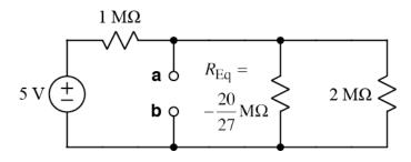
We could simplify further by computing the parallel value of the resistors on the right or taking a Norton equivalent of the voltage source and resistor on the left.
