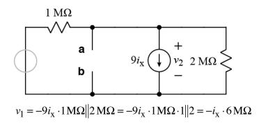
vi) Third, sum the two currents above and use Ohm's law to calculate the equivalent resistance of the dependent source as the voltage of the dependent source divided by the current of the dependent source:
