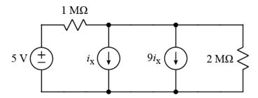
iv) Use superposition to calculate the voltage across the dependent source in terms of  $i_x$ . First, turn on the  $i_x$  source and turn off the  $9i_x$  source. Find the voltage across the dependent source (which is now an open circuit) in terms of  $i_x$ . We refer to this voltage as  $v_1$ :
