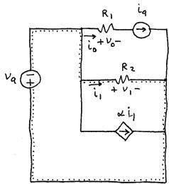
Only v-loop without current source is thru  $v_q$  and  $R_{Z_1}$  (dotted line).
