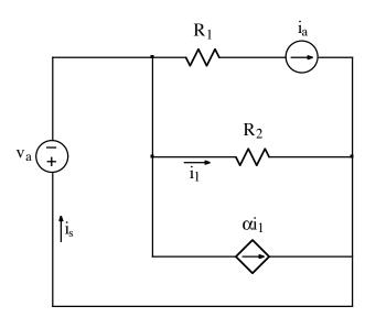
Derive an expression for  $i_s$ . The expression must not contain more than the circuit parameters  $\alpha$ ,  $i_a$ ,  $v_a$ ,  $R_1$ , and  $R_2$ . (Make sure to eliminate  $i_1$  from the answer.)
