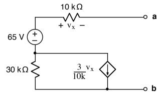
a) Find the Thevenin equivalent of the above circuit relative to terminals **a** and **b**.
