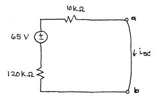
$i_{5c} = \frac{65V}{10K\Omega + 120K\Omega} = \frac{65V}{130K\Omega} = \frac{1}{2} mA$
