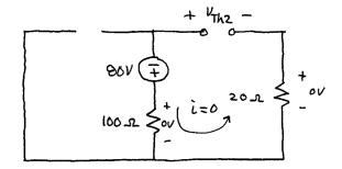
We have no current no V drop across R'\$. The 80V appears as  $-V_{Th2}$  across the terminals.  $V_{Th2} = -80V$ .
