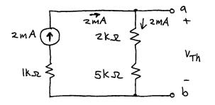
$v_{Th} = V_{a,b}$  open circuit = 2mA·(2kQ+5kQ)  $v_{Th} = 2mA \cdot 7kQ = 14V$  By: Neil E. Cotter
