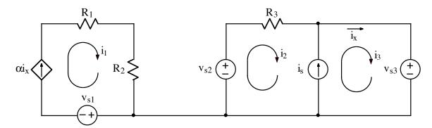
For the circuit shown, write three independent equations for the three mesh currents  $i_1$ ,  $i_2$ , and  $i_3$ . The quantity  $i_x$  must not appear in the equations.
