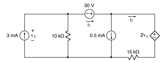
Use the mesh-current method to find  $i_1$  and  $i_2$ .
