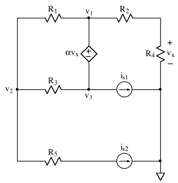
For the circuit shown, write three independent equations for the node-voltages,  $v_1$ ,  $v_{2}$ , and  $v_3$ . The quantity  $v_x$  must not appear in the equations.
