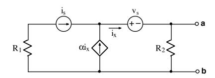
Find the Thevenin's equivalent circuit at terminals a-b.  $i_x$  must not appear in your solution. **Note:**  $\alpha \ne 1$ .
