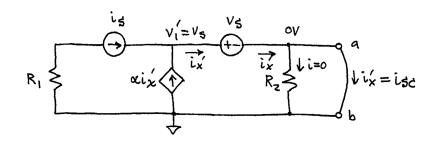
This is a different circuit than before. We have ov at a, (instead of  $V_{Th}$ ), and no current flows in  $R_2$  since it is bypassed by a wire. Also, isc =  $i_x$ .
