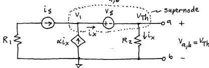
We first define ix in terms of node voltagest. Here, ix flows thru  $R_z$ . Thus ix =  $\frac{V_{Th}}{R_z}$ .
