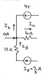
The voltmeter draws no current, and we have  $I_s = \frac{4}{3}A$  flowing into the node thru
