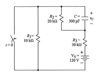
The switch has been open for a long time and is closed at t = 0.
