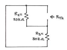
$$R_{Th} = R_2 || R_3 = 20 k_{\Omega} || 30 k_{\Omega}$$
