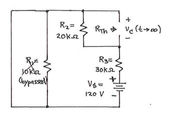
The voltage divider formula for ve now excludes  $R_1$ .  $V_c(t \rightarrow \infty) = -120V \cdot 20 k\Omega = -48V$   $20k\Omega + 30k\Omega$
