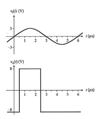
Using op-amps, power supplies, and resistors, draw a circuit to produce  $v_0(t)$  from  $v_i(t)$ . (Assume you have a function generator that produces  $v_i(t)$  for you to use.) Show all relevant information in your circuit, including positive and negative power supply voltages for op-amps. You may use only two power supplies in your design. You must generate other voltages you need from those two power supplies, (for example by using a voltage-divider).
