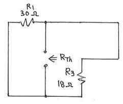
$$R_{Th} = 30\Omega || 18\Omega = 6\Omega \cdot 5|| 3 = 6\Omega \cdot \frac{15}{8} = \frac{90}{8}\Omega$$
