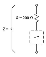
The total impedance of the above circuitry is  $Z = |Z|e^{j40^{\circ}}$ . We don't know the magnitude of Z, but its phase angle is  $+40^{\circ}$ . Z is made of a  $200\Omega$  resistor in series with one other part. What is that part? Give the type and value of the part, and draw the combination.
