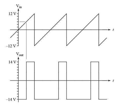
Using op-amps, power supplies, and resistors, draw a circuit to produce  $V_{out}$  from  $V_{in}$ . (Assume you have a function generator that produces  $V_{in}$  for you to use.) Show all relevant information in your circuit, including power supply voltages for op-amps.
