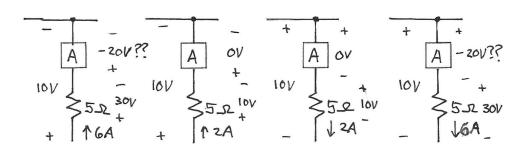
The voltage drop across the 52 resistor is given by Ohm's law: V = IR. The voltage drop across A plus the voltage drop across the 52 resistor in B equals 10V. This means we have either -20V across A or OV across A.
