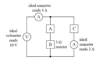
If box A contains a resistor, find the value of that resistor.
