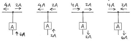
The current flowing in A is chosen to make the sum of currents at the node equal zero.
