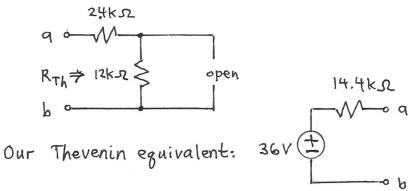
b) When R<sub>L</sub> is not present, there is no current in the 2.4 ks resistor and no power consumed by it. The power supplied by the current source is the power consumed by the 12 ks resistor. From part (a), we know that 3 mA flows in the 12 ks, so we have the power from I<sup>2</sup>R:
