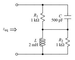
Find the numerical value of the equivalent impedance,  $z_{eq}$ , for the circuit. Frequency  $\omega = 1$  Mr/s. Express your answer in both rectangular and polar form.
