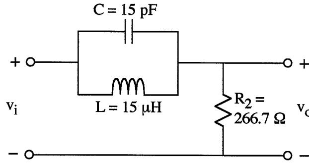
For the band-reject filter shown above, calculate the following quantities:
