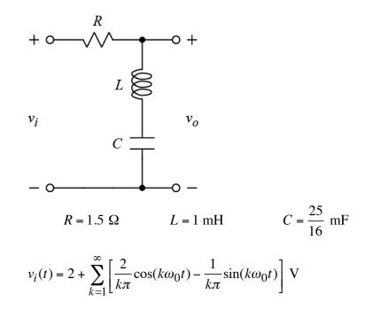
Write the time-domain expression of the first harmonic (i.e., k = 1) of  $v_0(t)$ . Note:  $\omega_0 = 3.2$  k r/s for the Fourier series.
