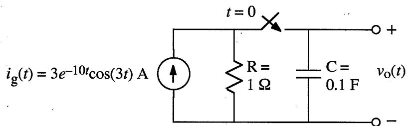
**Note:** The initial voltage on the capacitor is  $v_C(t = 0^-) = 3$  V measured with + on top.
