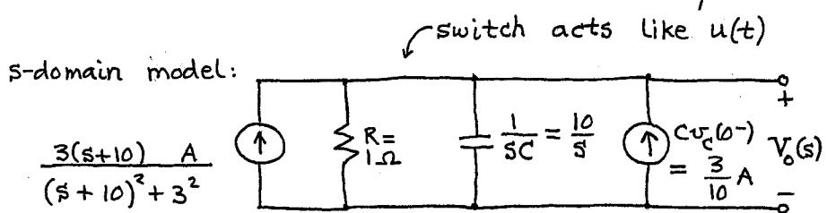
The output voltage is the total current times the total parallel resistance.
