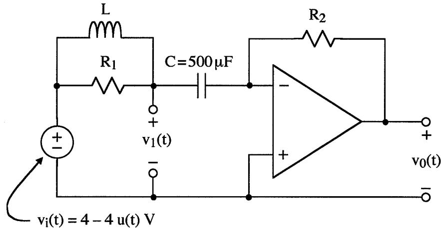
The Laplace transform of  $v_0(t)$  for the above circuit is as follows:
