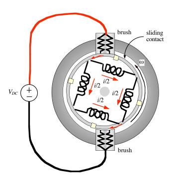
The maximum current still flows in the coils, but a gap between the sliding contacts is about to pass under the brush.
