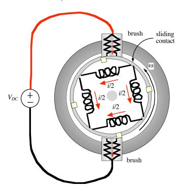
As the top-left sliding contact breaks contact with the brush, all the current for the coil on the left now flows through the top coil. Complete reversal of current has been achieved, and the next quarter cycle begins.
