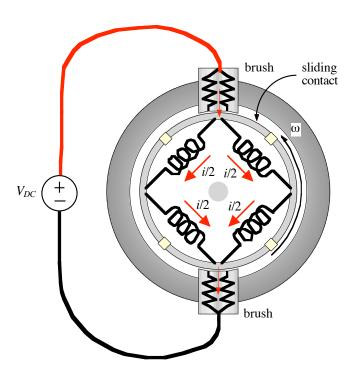
The above illustration shows a DC motor with four coils attached to four sliding contacts that make contact with two brushes. As the rotor moves, the directions of currents will eventually be reversed. We follow this process through approximately one-fourth rotation.
