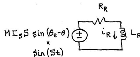
The response of the circuit will be sinusoidal and at the same frequency as the source.
