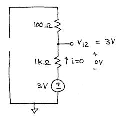
We sum  $V_{11}$  and  $V_{12}$  to get  $V_1$ .  $V_1 = V_{11} + V_{12} = -6V + 3V = -3V$ For  $v_0$  to be -12V at  $t=t_0^-$  we must have  $V_2 > V_1$ . This condition is satisfied by placing either an L or R in box **a**. If we have an L in box **a**, then it will act like a wire at  $t=t_0$ , making  $V_2$ equal to 0V. If we an R in box **a**, however, we will have a V-divider:
