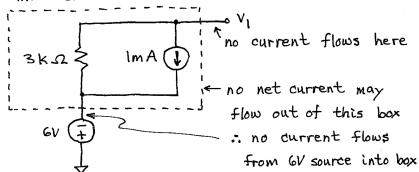
We have  $V_1 = -6V - 1 \text{ mA} \cdot 3 \text{ k} \Omega = -9V$ . Note that the 1 mA must flow through the 3 k  $\Omega$  resistor since no current flows into the op-amp.
