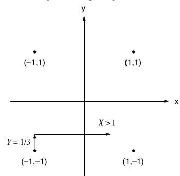
For the received signal to be closer to (1, -1) than to (-1, -1), the value of *X* must be greater than 1, as the diagram shows. Thus, we find the conditional probability f(x | y = 1/3) and determine the conditional probability that X > 1.
