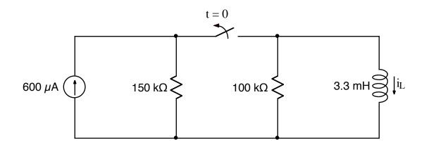
After being closed for a long time, the switch opens at t = 0. Find  $i_L(t)$  for t > 0.
