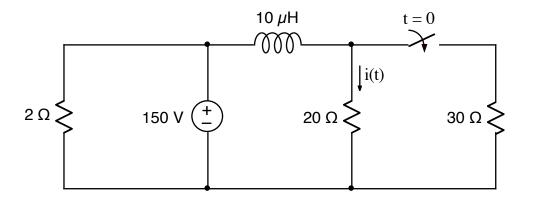
After being closed for a long time, the switch closes at t = 0.
