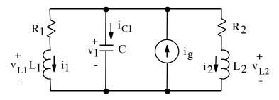
The equation for  $v_{L1}$  must come from a voltage loop, and the voltage loop on the left will suffice in this case. We use Ohm's law to express the voltage across  $R_1$ :
