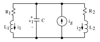
Third-order circuit.  $i_g(t)$  switches from  $-i_0$  to  $i_0$  at t = 0.
