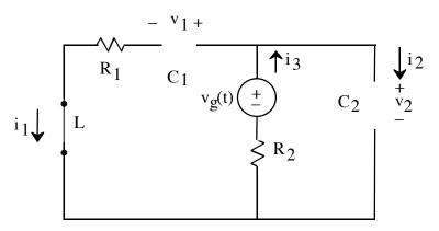
Because the inductor is in series with an open circuit, the inductor current will be zero. Similarly,  $i_2 = 0$ , and it follows that  $i_3 = 0$ . Thus, there is no current in any of the resistors, and no voltage drop across any of the resistors. Consequently,  $v_g(t)$  appears across  $C_1$  and across  $C_2$ . At time t = 0,  $v_g(t) = -v_o$ .
