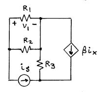
Careful inspection reveals that R<sub>1</sub> and R<sub>2</sub> are in parallel and is flows thru R, and R<sub>2</sub>.
