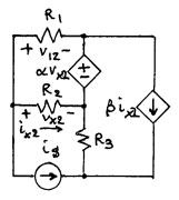
We can always use node-voltage. Putting a reference in the center is convenient.
