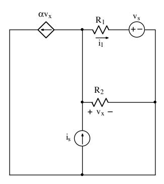
Using superposition, derive an expression for  $i_1$  that contains no circuit quantities other than  $i_s$ ,  $v_S$ ,  $R_1$ ,  $R_2$ , and  $\alpha$ , where  $\alpha > 0$ .
