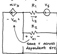
The dependent source is equivalent to  $Reg = \frac{V}{i} = \frac{V_{x1}}{\alpha V_{x1}} = \frac{1}{\alpha}$ .
